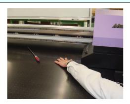
Do not put your hands on the carriage moving path when the printer power is ON.
