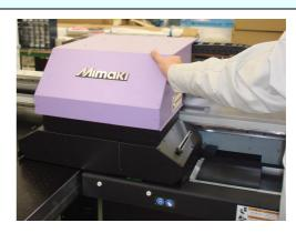
Do not move the carriage manually while the carriage operates (during printing and cleaning).
