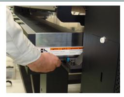
Do not put your hands into the gap between the Y bar and the table with the power is ON.
