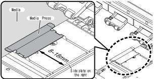
Media press position: 8 to 18 mm from the side plate on the right. (For the variation of the inside diameter of media roll, it ranges as above.)
